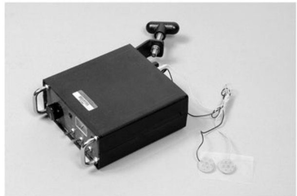
Figure 1 The connectors, on the pediatric ECG pads manufactured by Kendall, are both electrically and mechanically compatible with several of Neuro Technology's variable-current train-of-four stimulators. This combination is useful in assessing pediatric neuromuscular blockade.
