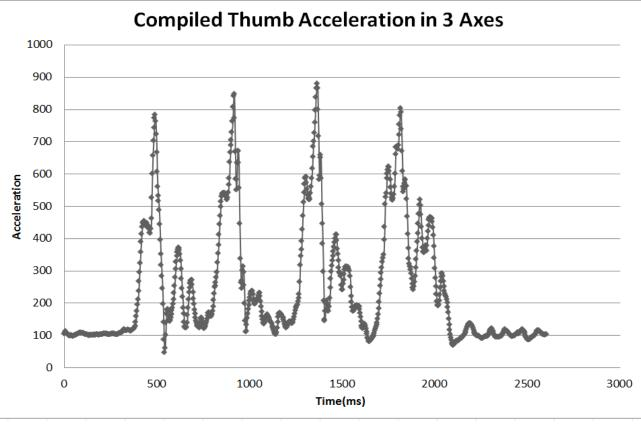
The root mean square composite of the 3 axes creates a consistent baseline regardless of clip
