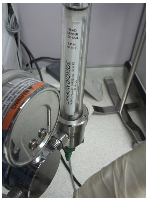
FIGURE 2. A green oxygen Christmas tree adapter inappropriately attaches onto a carbon dioxide flow meter.
