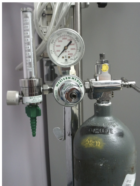
FIGURE 1. A green oxygen Christmas tree adapter inappropriately attaches onto a carbon dioxide flow meter.
